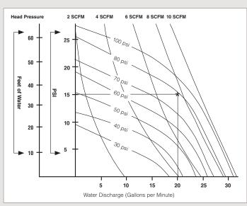
At 80 psi air pressure and 15 psi fluid pressure, an AP-30 pump operates at 20 gpm.
