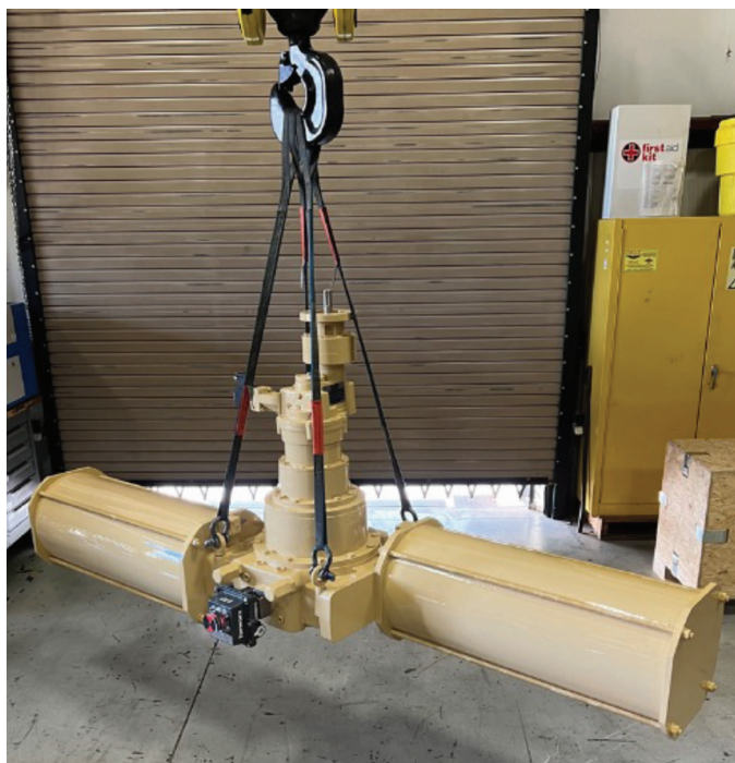
Figure 3.2: Using the lifting eyes for the Limitorque fail-safe actuator RSDS
