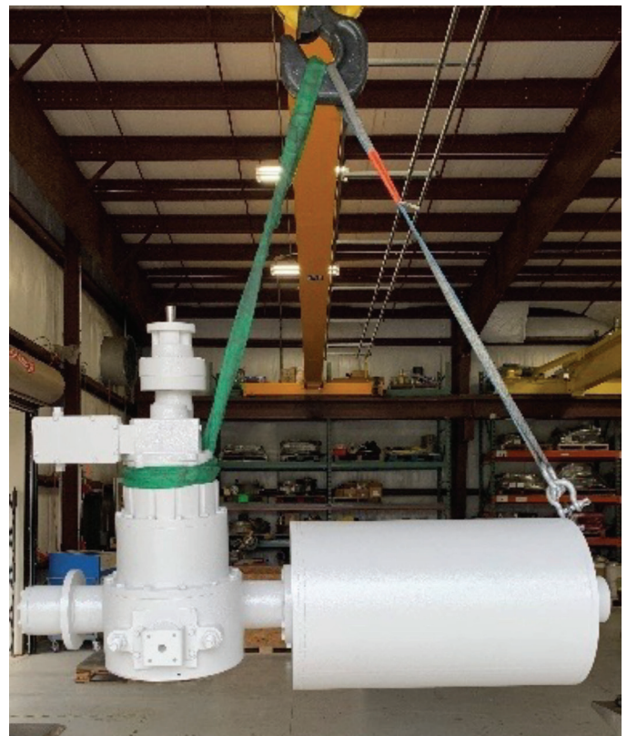
Figure 3.1: Using the lifting eyes for the Limitorque fail-safe actuator RS
