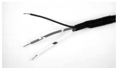
Figure 3.6 - Applying heat shrink tubing
