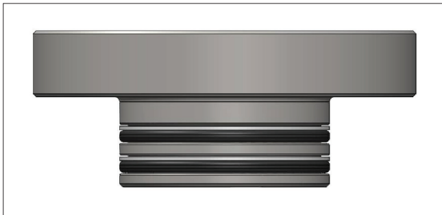
Figure 5: Top Cover with O-Rings and Back-up rings
