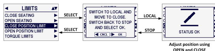
Figure 4.16: Calibrating electrical operation
