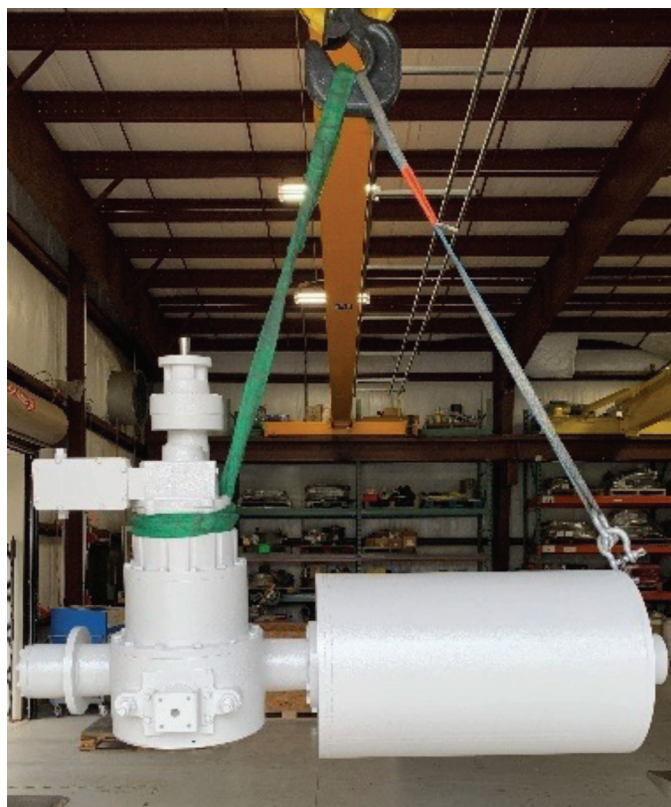
Figure 3.1: Using the lifting eyes for the Limitorque fail-safe actuator RS
