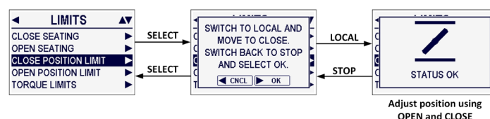
Figure 4.17: Calibrating handwheel operation
