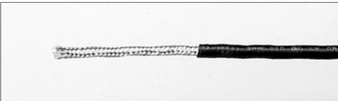
Figure 4.5: Removing the outer plastic jacket
