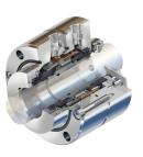
Eliminate fugitive emissions and handle reverse pressurization upsets with this face-to-back configured, dual pressurized seal that complies with API 682, Arrangement 3.
